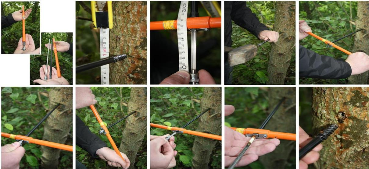
Figure 2: The tree coring procedure using a SUUNTO borer. *Photos by M. Algreen.*
