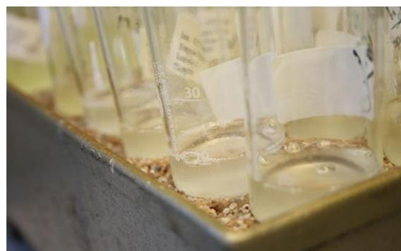
Figure 4: a) Decay of the tree cores in HNO<sub>3</sub> on a sand bath.
